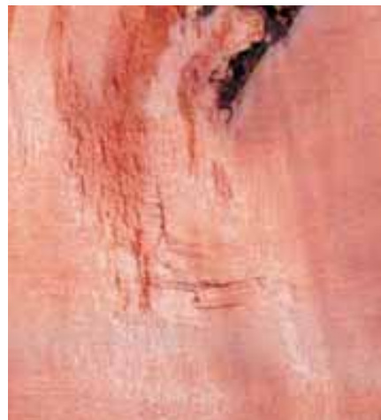
Photo: Tear-out often occurs on areas of wild grain when using a conventional cutter on a planer or thicknesser
